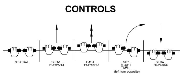
From neutral position, gently push both drive levers forward. To increase speed, move levers farther forward.
